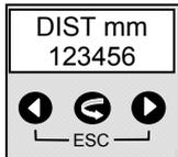
the text “DIST mm” or “DIST INCH” (depending on unit selected) and the actual measured value are displayed on the screen.
