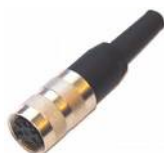
CON011: mating connector for self assembly IP40, 5 pole, cable diameter 4...6 mm
